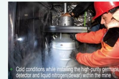
Cold conditions while installing the high-purity germanium detector and liquid nitrogen (dewar) within the mine
